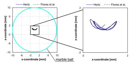
Fig. 12 *xz*-trajectory of the contact points of the marble ball when using the Hertz law and the Flores et al. model
