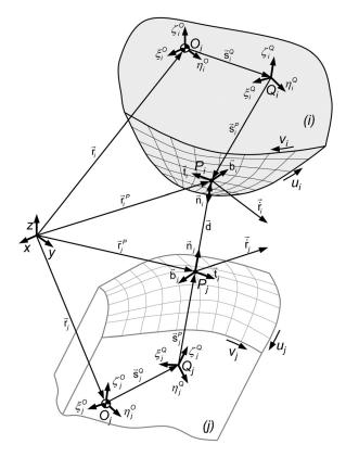
Fig. 4 Representation of two generalized contact surfaces
