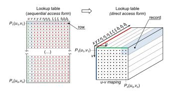
Fig. 3 Schematic representation of the lookup table reshuffle of a surface defined with 100 points that are stored in 25 records
