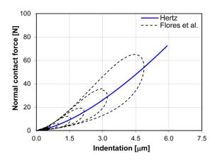
Fig. 14 Force-indentation relations of the contact between the marble ball and the cup during the first 0.1 s of simulation
