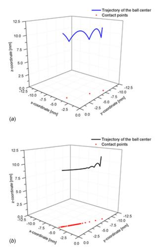
Fig. 15 Trajectory of the ball center and the relative contact points during 0.1 s of simulation using two contact force approaches: (a) Hertz law; (b) Flores et al. model
