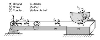
Fig. 9 Initial configuration of a slider-crank mechanism with a cup (body 5) on the top of the slider and a marble ball (body 6)
