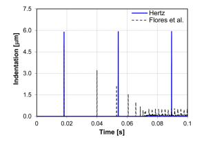
Fig. 13 Contact indentation between the marble ball and the cup during the first 0.1 s of simulation
