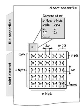
Fig. 6 Structure of a direct access file of a parametric representation of a surface with 100 points
