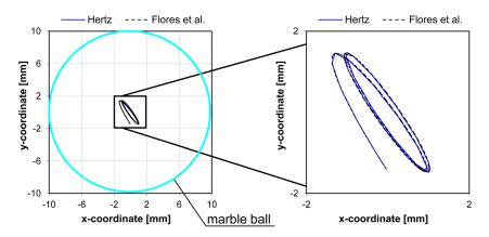
Fig. 11 *xy*-trajectory of the contact points of the marble ball when using the Hertz law and the Flores et al. model
