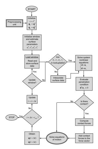
Fig. 8 Computational algorithm proposed to deal with 3D contact problems in multibody systems
