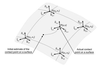
Fig. 5 Schematic representation of the bilinear interpolation for a surface described by four points
