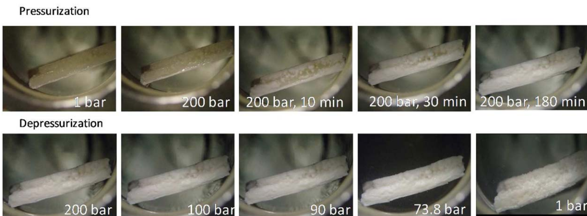
Figure 3. Effect of pressurization and depressurization on foaming process for the system SPCL + TA-glucose (1:1).
