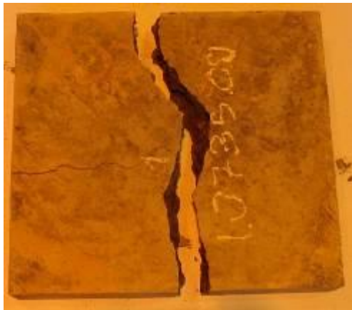
(a) Concreto convencional (CCV)
