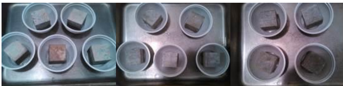
Figure 6: Specimens of the cement based mortars in cycle 0: C32.5N500-0PCM, C32.5N500-40PCM and C32.5N500-F-40PCM, from the left to right.
