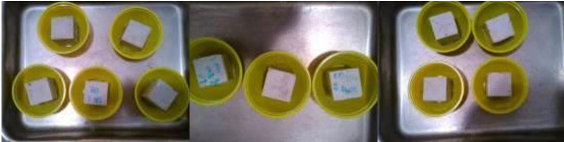
Figure 8: Specimens of the aerial lime based mortars in cycle 0: CA500-0PCM, CA800-40PCM e CA800-40PCM-F, from the left to right.
