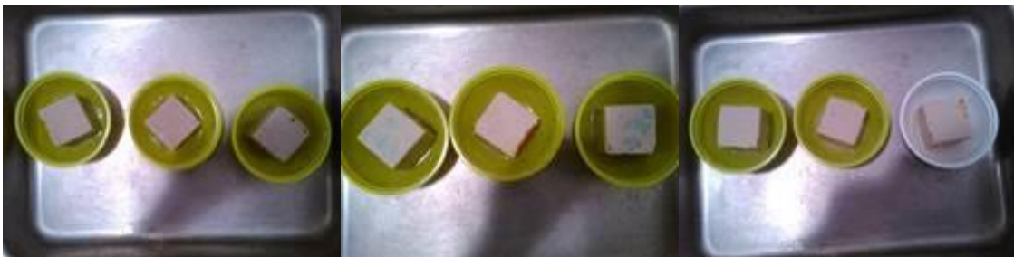
Figure 9: Specimens of the gypsum based mortars in cycle 0: G500-0PCM, G500-40PCM e G500-40PCM-F, from the left to right.
