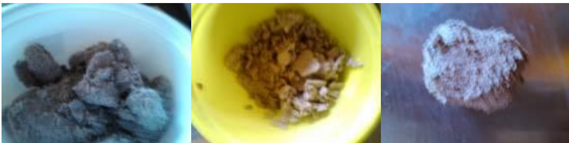
Figure 12: Final aspect of the specimens of the hydraulic lime based mortars in the cycle 56: CH500-0PCM, CH500-40PCM e CH500-40PCM-F, from the left to right.
