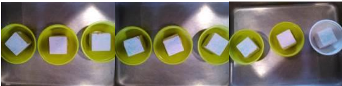
Figure 14: Final aspect of the specimens of the gypsum based mortars in the cycle 56: G500-0PCM, G500-40PCM e G500-40PCM-F, from the left to right.
