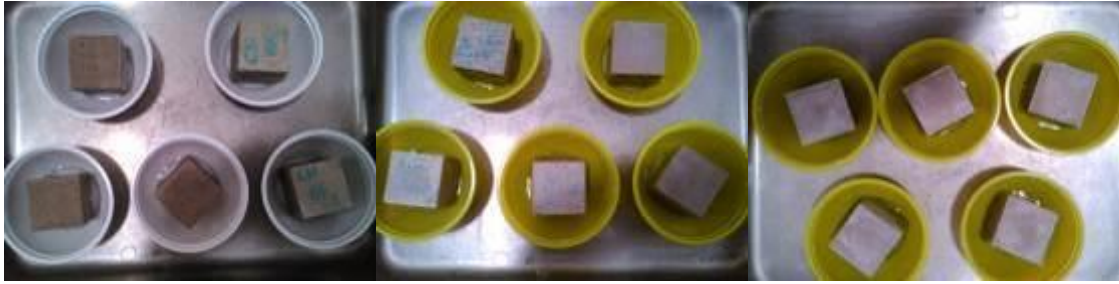
Figure 7: Specimens of the hydraulic lime based mortars in cycle 0: CH500-0PCM, CH500-40PCM e CH500-40PCM-F, from the left to right.
