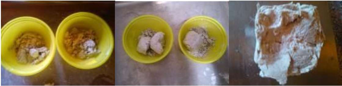
Figure 13: Final aspect of the specimens of the aerial lime based mortars: CA500-0PCM in the cycle 27, CA800-40PCM in the cycle 6 e CA800-40PCM-F I the cycle 56, from the left to right.
