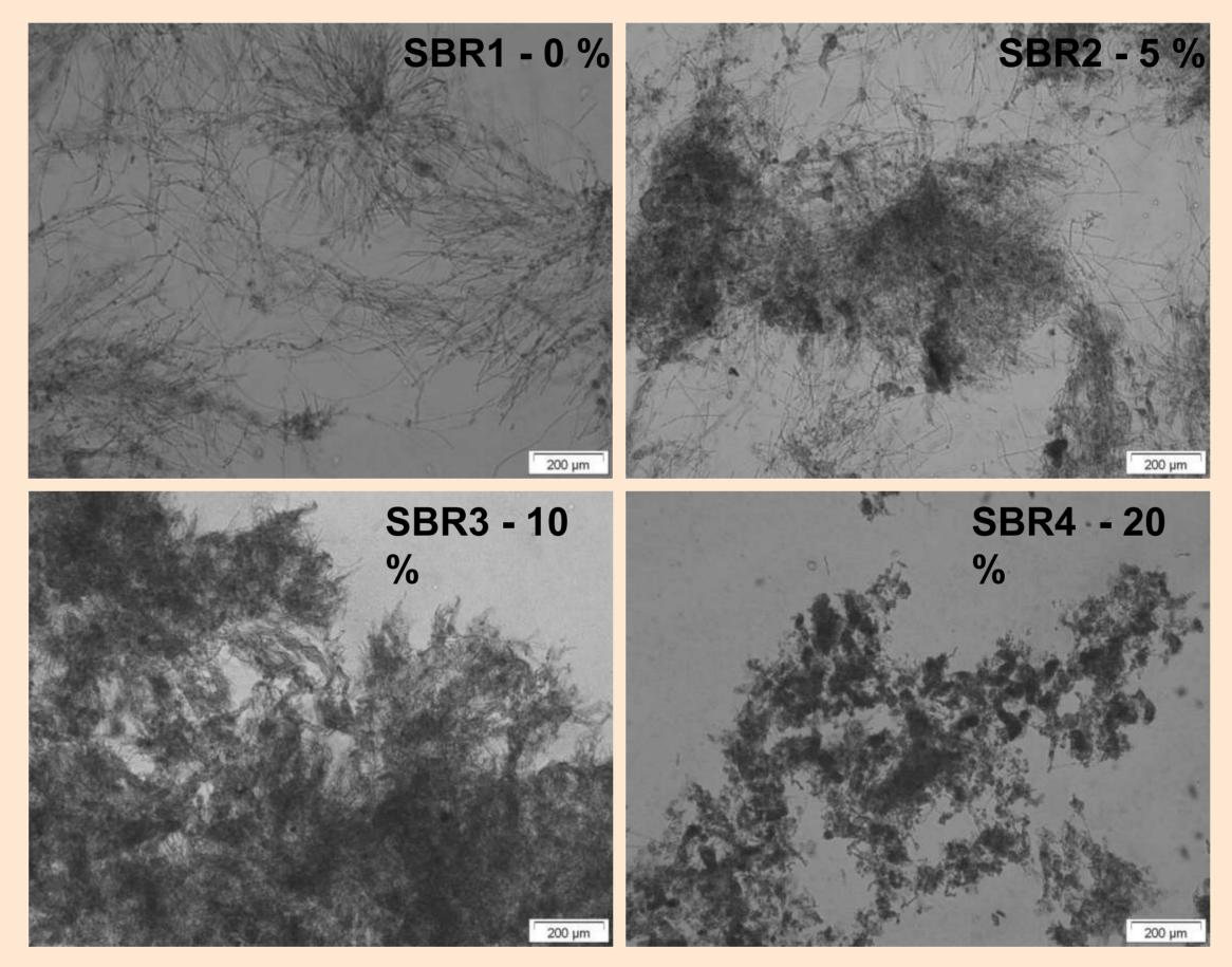
→ Filamentous bulking was observed in SBR1 and SBR2. In SBR3 and SBR4 filamentous bulking did not occur.
