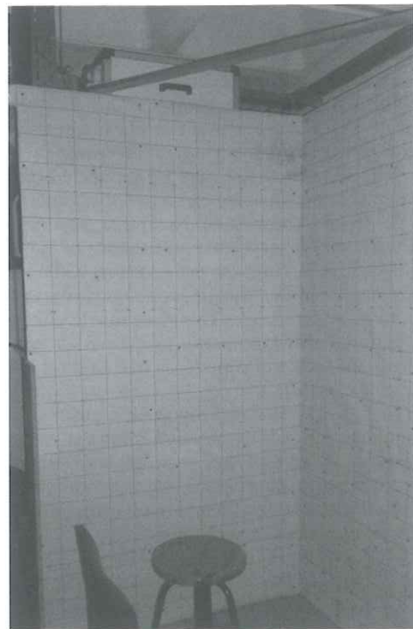
Figure 1. Stationary anthropometer with 1200 × 1500 × 2100 (depth, width, height), in mm.
