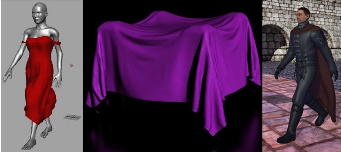
Figure 1.4: Examples of spring/mass models via particle system approach (from left to right): Maya nCloth simulation, Blender's built in cloth dynamics and Havok cloth simulation. [80-82]
