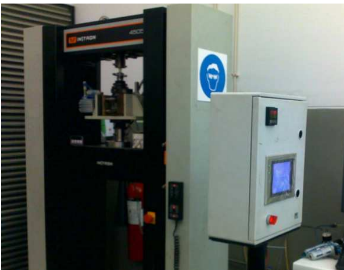
Figure 1. Testing apparatus for coefficient of friction measure.
