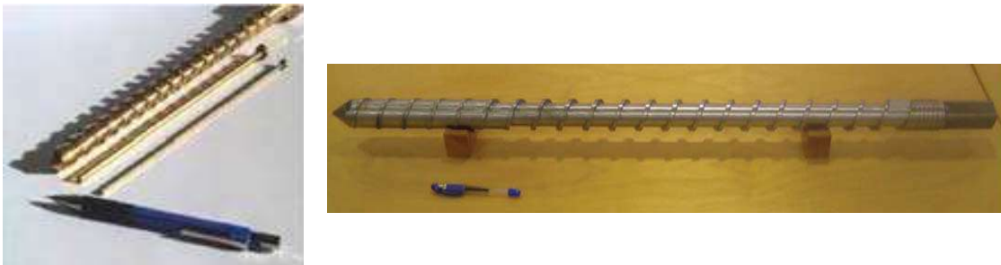
Figure 2.14 - Comparison of dimensions between screw and injection plungers for \mu IM (left) and a screw for conventional injection molding (right) [113].
