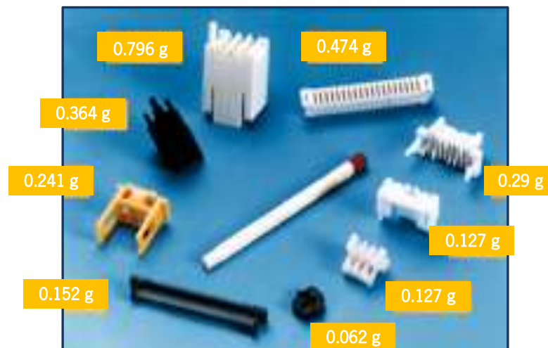
Figure 2.16 - Examples of microparts with weight in the range of milligrams [141].
