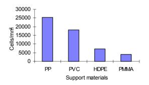
Fig.1 - Results of adhesion tests performed, expressed by the number of bacteria per square mm of the polymer surface.
