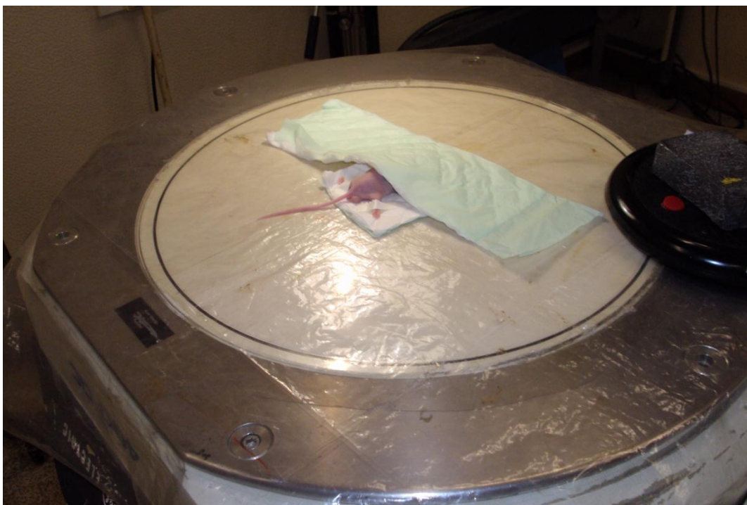
Figure 39. Positioning of balb/c nu/nu mouse in the detector of the gamma-camera (GE 400 AC).
