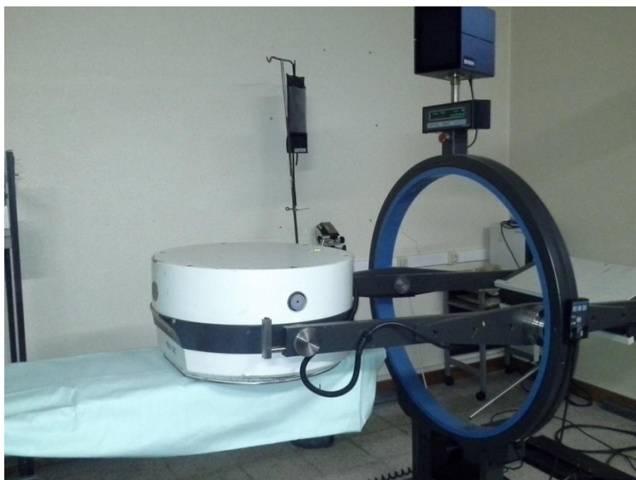
Figure 37. Gamma-camera (GE 400 AC) coupled with a low energy, parallel hole and high resolution collimator.
