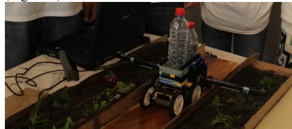
Figure 2 - The irrigation system.
