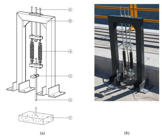
Figure 1. Proposed system: (a) Schematic representation; (b) Prototype used in situ testing.
