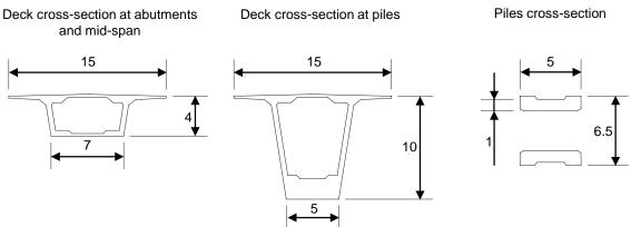
Figure 5. New bridge over Dão River near Coimbra, Portugal (all dimensions are in meters).
