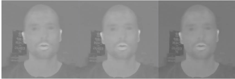
Figure 19 - Y (image on the left), Cb (image in the center) and Cr channels (image on the right) from the YCbCr frame
