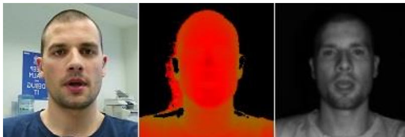
Figure 16 - Images collected from the RGB (left), depth (center) and IR (right) streams
