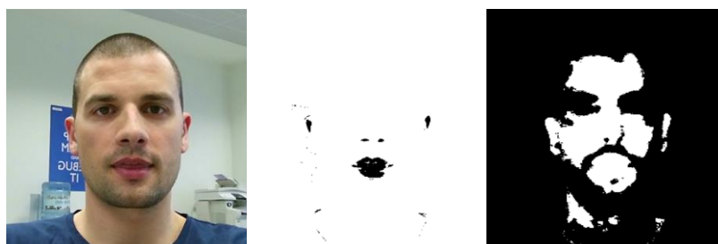
Figure 24 - RGB frame (left image), processed green channel (center image) and processed Cr channel (right image) showing the effacement of the inner contour due to the visibility of the tongue during the word "Calendário"
