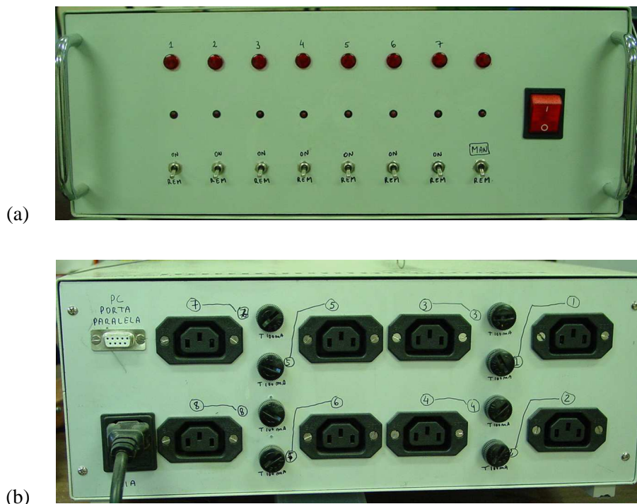
Figure C.1.: Valve controller (a) front panel and (b) rear panels
