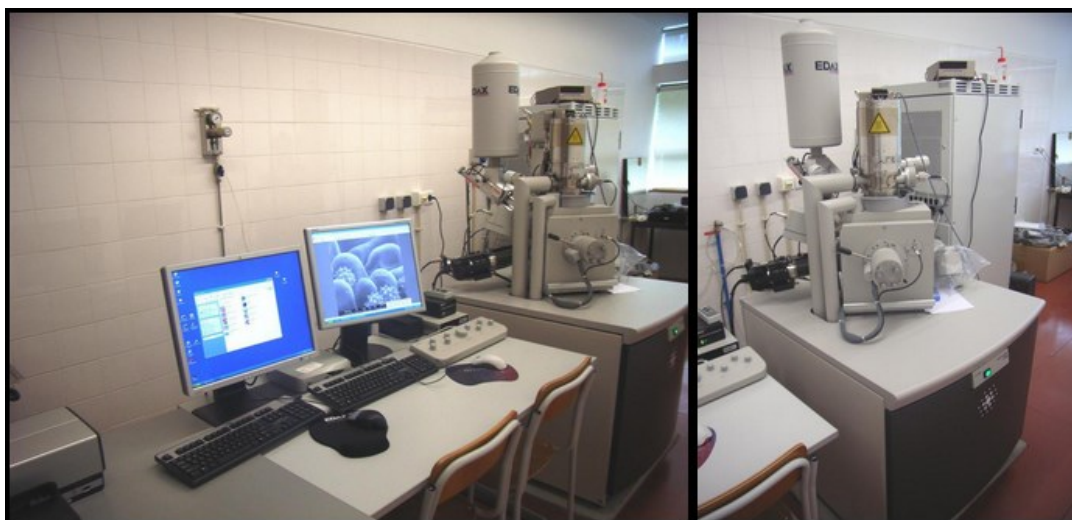
Figure 16. Photos of EDS and SEM equipment, FEI Nova (FEG/SEM); EDAX - Pegasus X4M (EDS/EBSD) [38]
