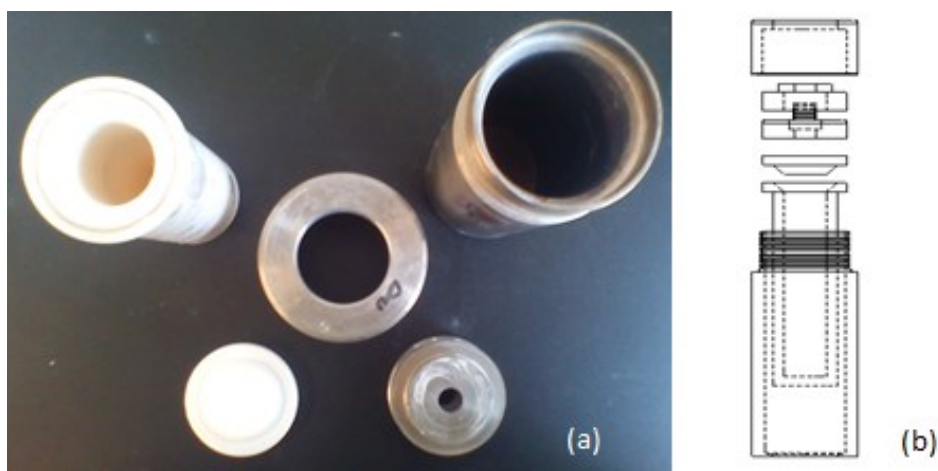
Figure 9. Autoclave used for stannosilicate hydrothermal synthesis; (a) autoclave components (photo) (b) assembly.
