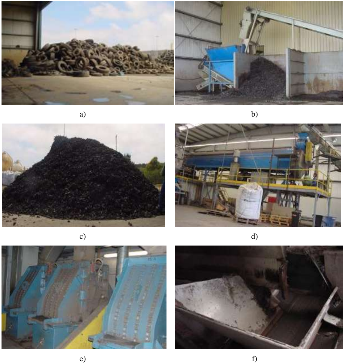
Figure 1. Overview of the industrial process to transform tires in fibres for use in the reinforcement of concrete: a) waste tires to be recycled, b) waste tires transformed in pieces of rubber, c) stock of pieces of rubber, d) cryogenic tunnel to put tires in the glassy state, e) tunnel hammers to break the pieces of rubber in glassy state and f) the fibres are separated by magnetic and collected in a container
