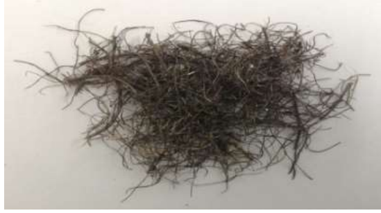
Figure 2. Recycled steel fibres extracted from wasted tires
