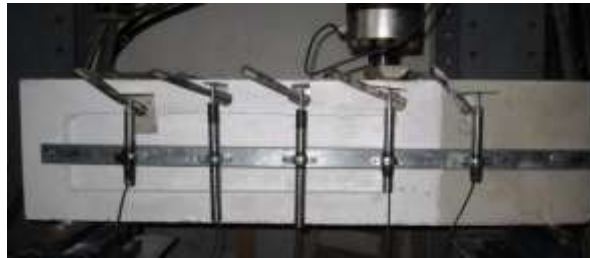
Figure 14. Beam configuration, test setup and position of the LVDTs (dimensions in mm)
