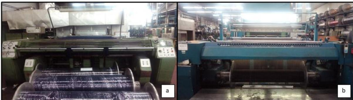
Figura 20 - (a) Engomadeira 1 (b) Engomadeira 2
