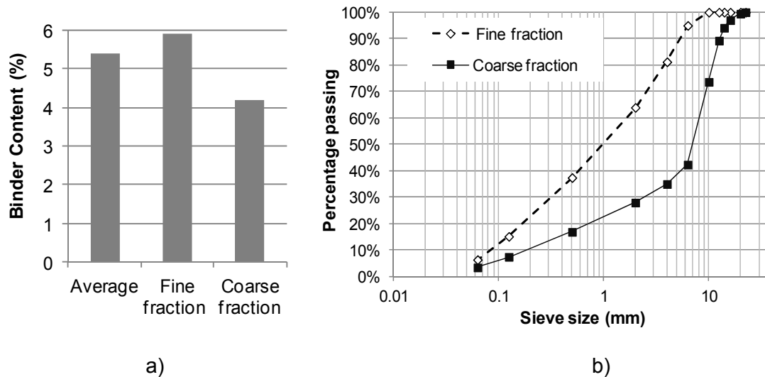
Figure 2 Binder content (a) and particle size distribution after incineration (b) of the different RA fractions
