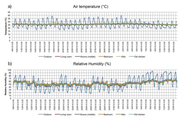
Figure 12. Case study 2 performance during summer season. (a) Indoor and outdoor air temperature profile; (b) Indoor and outdoor relative humidity profile.
