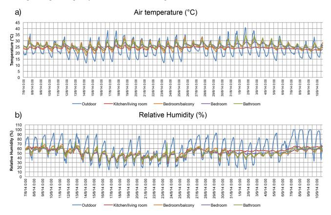
**Figure 8.** Case study 1 performance during summer season. (**a**) Indoor and outdoor air temperature profile; (**b**) Indoor and outdoor relative humidity profile.
