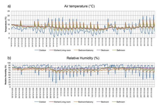
**Figure 10.** Case study 1 performance during winter season. (a) Indoor and outdoor air temperature profile; (b) Indoor and outdoor relative humidity profile.
