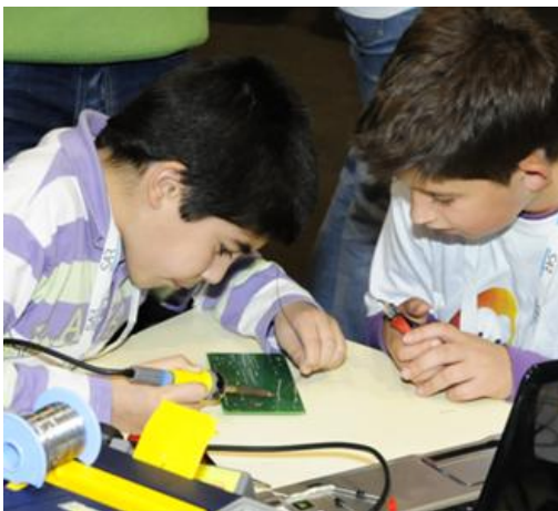
Fig. 8. Two youngsters working on soldering the electronic components, one is soldering and the other cuts the excess of the component pins
