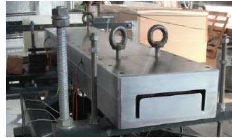
a) Die mounted on the pultrusion equipment
