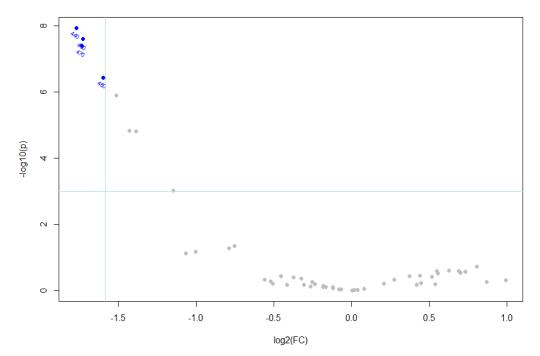
Figure 3: Volcano plot analysis (Fold change threshold = 2 and p  $\leq$  0.001). The larger magnitude fold changes and the higher statistical significance refer to wavelengths between 440-470 nm. (blue symbols).
