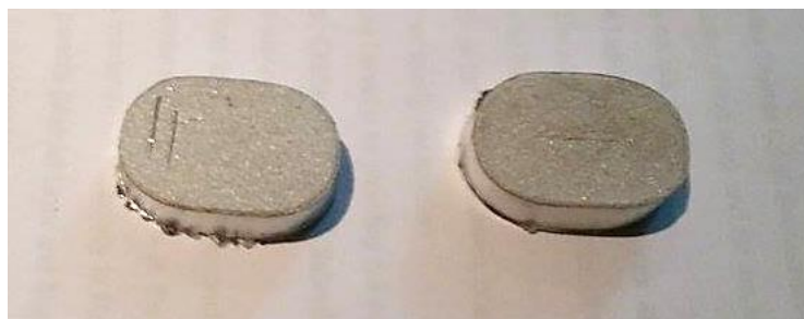
Figure 3.20 - Tested samples (Zn-Al15 – Sn-Cu3) with and without the scratches.
