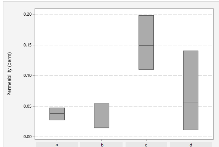
Figure 3.19 - Permeability values for a) Zn-Al15 (225 \mu\text{m} ) – Sn-Cu3 (145 \mu\text{m} ), b) Zn-Al15 (275 \mu\text{m} ) – Sn-Cu3 (325 \mu\text{m} ), c) Zn-Al15 (225 \mu\text{m} ) – Sn-Cu3 (225 \mu\text{m} ) and d) Zn-Al15 (325 \mu\text{m} ) – Sn-Cu3 (325 \mu\text{m} ).
