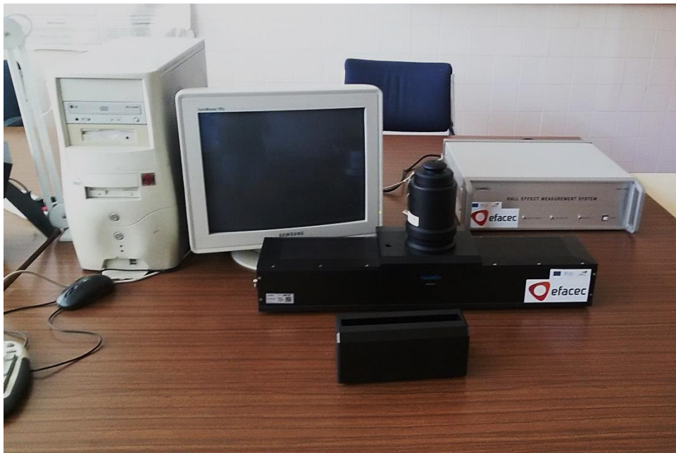
Figure 2.14 - HMS-5300 Hall Effect Measurement System (Dept. Physics, Univ. Minho).
