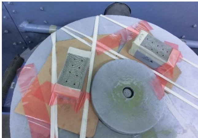
Figure 2.9 – Plastic cases in the substrate of the spraying machine (Vishay).
