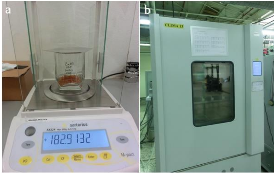
Figure 2.12 – a) Weight of the test dishes (Vishay); b) Climatic chamber (Vishay).
