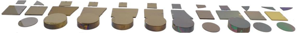
Figure 4.13 Films obtained with the variation of the reactive gas flow in the different substrates (silicon, glass and steel) – RG# series
