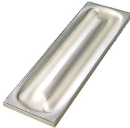
Figure 3.4 Non-uniform erosion of the target – 'race track'[63]
