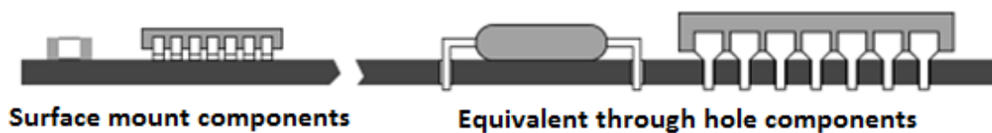
Figure 5. Schematic representation of the types of components that exist, SMD and TH [8].
