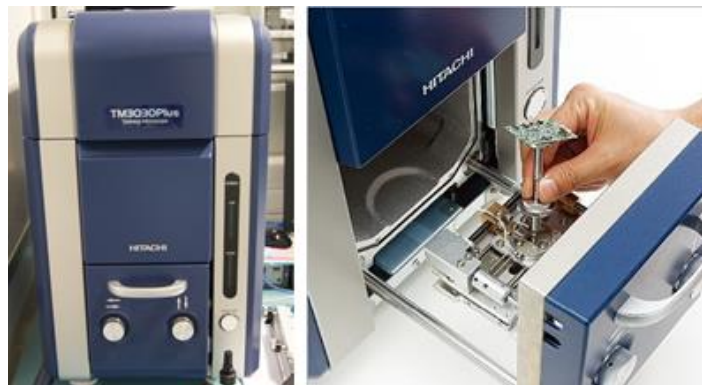
Figure 34. Bosch Car Multimedia scanning electron microscopy (SEM) and Energy dispersive X-ray spectroscopy (EDS), Hitachi TM3030Plus.
