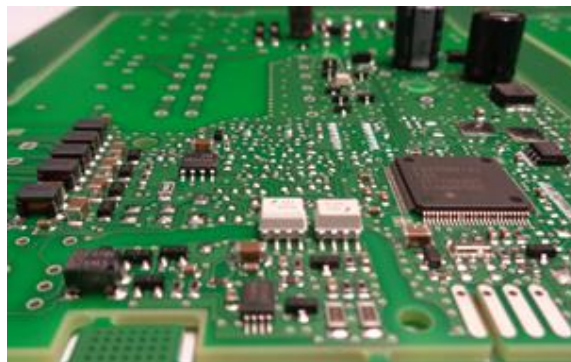
Figure 1. Printed Circuit Board, SolarA after Reflow and Radial process.
