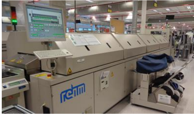
Figure 24. Bosch Car Multimedia Reflow oven, REHM, utilized to SolarA production.
