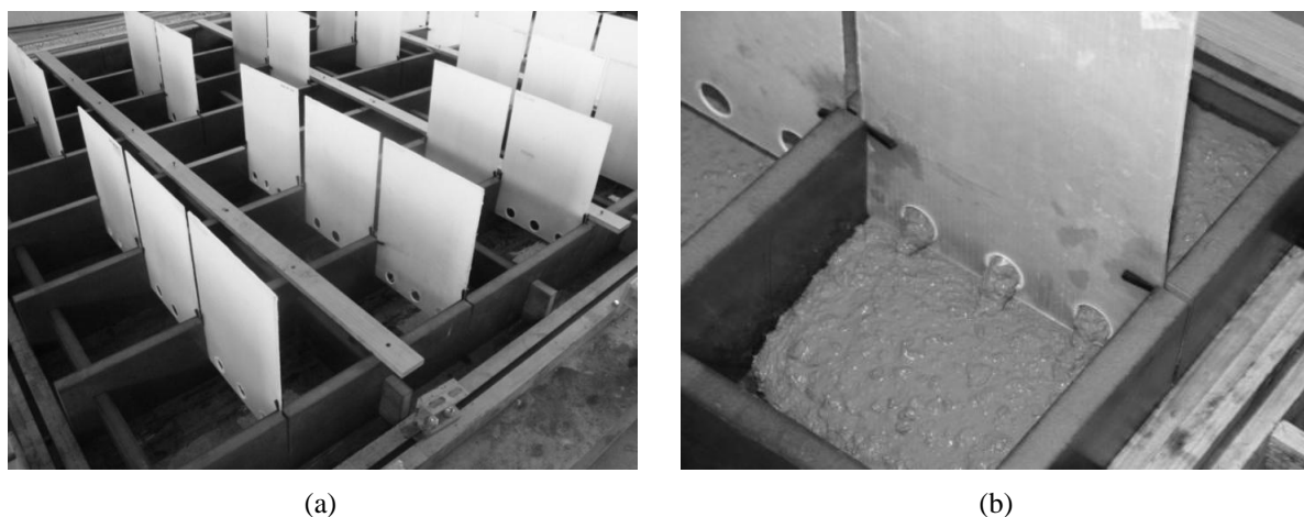
Figure 136: Production of pull-out specimens: (a) overall view of formwork; (b) pouring of 3H-MU4-SCC specimen.
