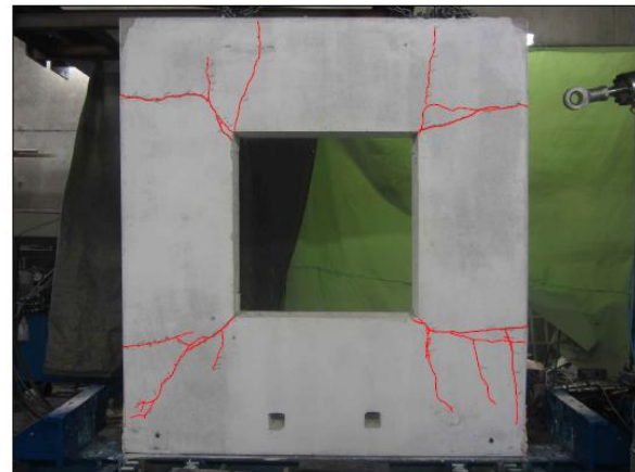
Figure 183: Typical cracking pattern of prototypes with opening (OP).
