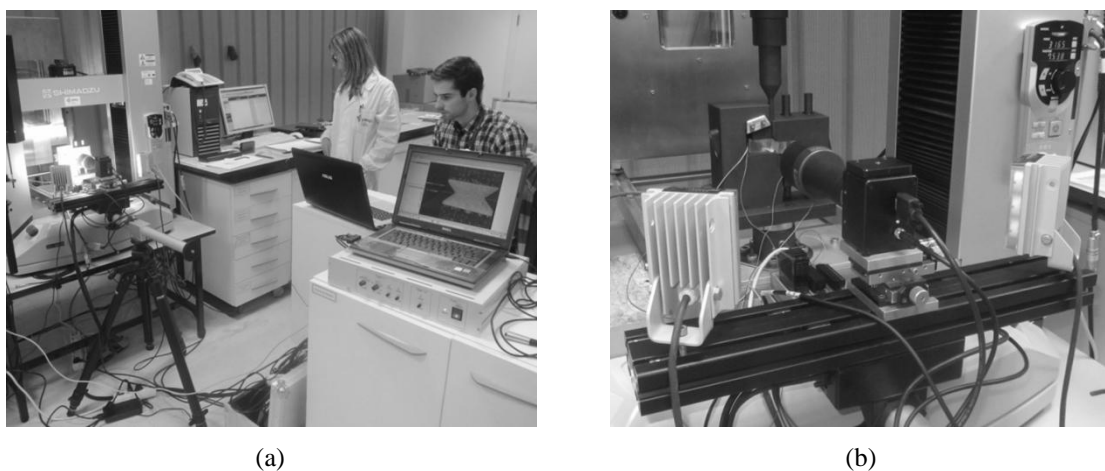
Figure 63: Test setup: (a) overall view; (b) detailed view of specimen positioned in the fixture and the position of the camera..
