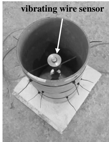
Figure 44: Detail of the vibrating wire sensor prior to the casting of specimen for TDC test.
