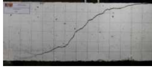
b) Crack pattern at failure load of the OS-R beam
