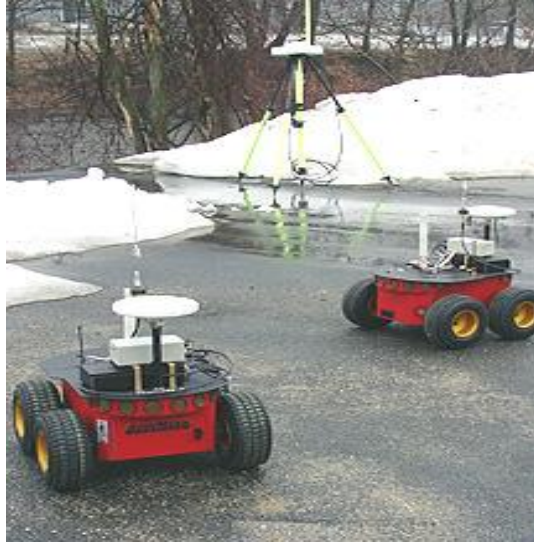
Figure 5 – ActivMedia Mobile Robot - PIONEER 3-AT [W28]
