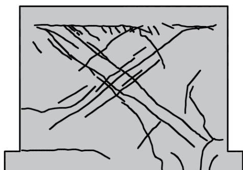
Figure 10: Final cracking pattern of the specimen retrofitted with commercial TRM.
