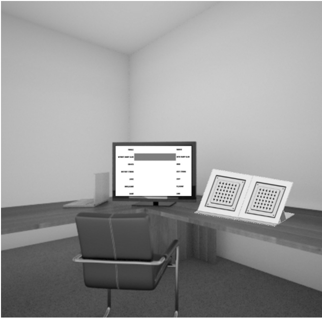
Fig. 3. Set-up of the experiment. The participant was seated in front of a touch screen and the two key platforms. In the touch screen, all seven pairs of Kansei words were displayed, and the pair currently under evaluation was highlighted with a green bar. The participant should touch a point along the scale, depending on his or her evaluation of the key.
