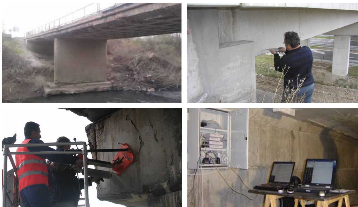
Fig. 16. Main approaches in damage detection: visual inspection, non-destructive testing, probing and structural health monitoring.
