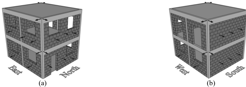
Figure 6: Accelerometers setup (Model 1): (a) North and East facades; (b) South and West facades.
