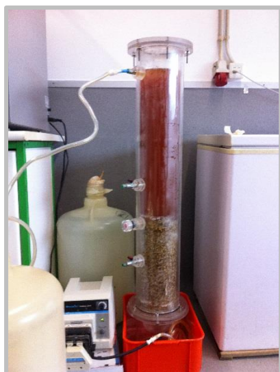
Figure 6.1. Pilot scale installation for a) the growth and formation of the S. equisimilis biofilm on vermiculite at room temperature; b) biodegradation and biosorption assays of diethylketone and Ni^{2+} or diethylketone and Cd^{2+} .
