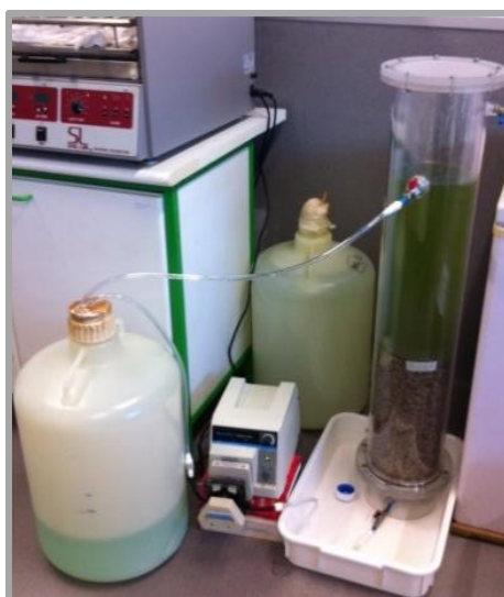
Figure 6.1. Pilot scale installation for a) the growth and formation of the S. equisimilis biofilm on vermiculite at room temperature; b) biodegradation and biosorption assays of diethylketone and Ni^{2+} or diethylketone and Cd^{2+} .
