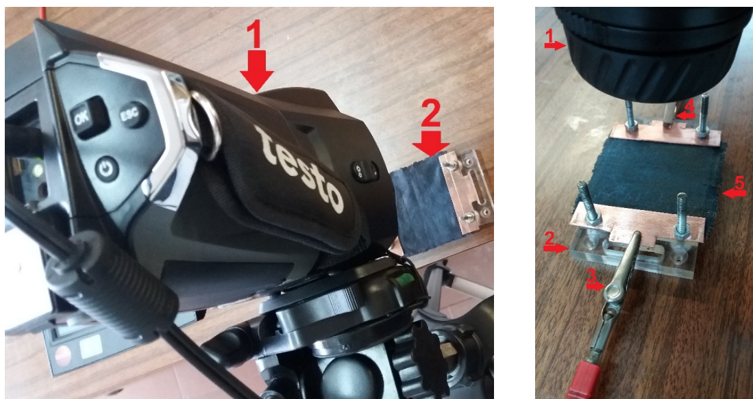
Fig. S8 Joule heating experiment set-up. Left: Thermal camera (1) and fabric holder with two copper electrodes (2) configuration; Right: Thermal camera lens (1), fabric holder (2), copper anode (3), copper cathode (4) and conductive fabric (5).
