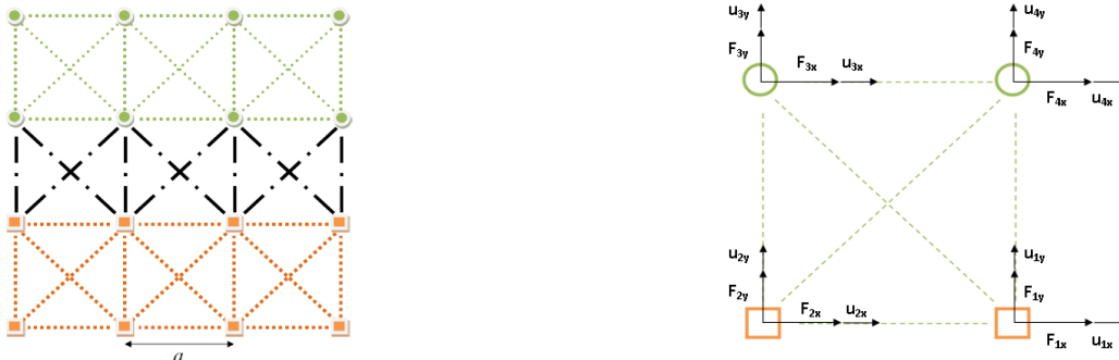
(A) A model for materials A and B in contact. (B) Applied forces and displacements at each node.
