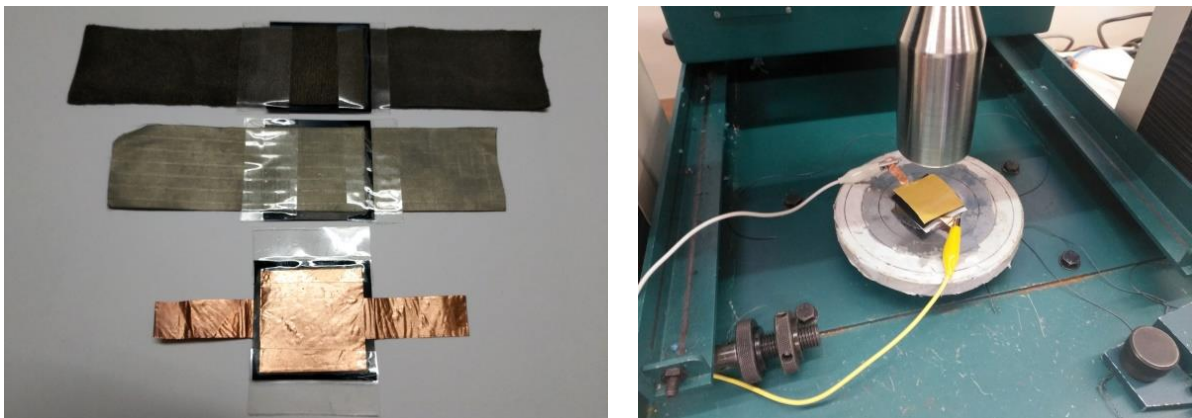
Figure 1 (left): Sensors with conductive knitted stretch fabric (upper), conductive woven ripstop fabric (middle) and copper tape (lower) as electrodes. (right) Compression test setup
