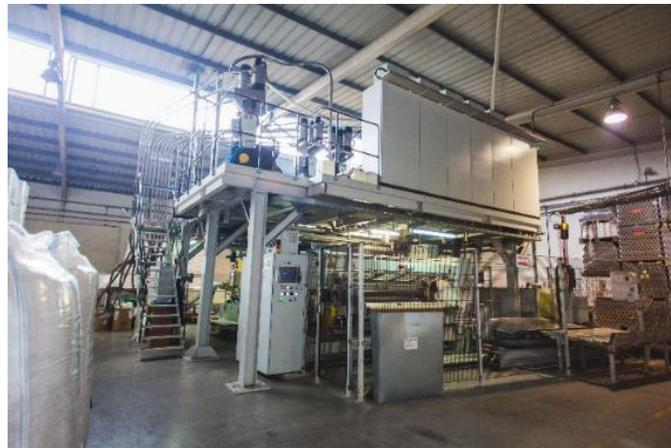
Figura 21 - Extrusora “Cast1” (Rembalcom, 2015)
