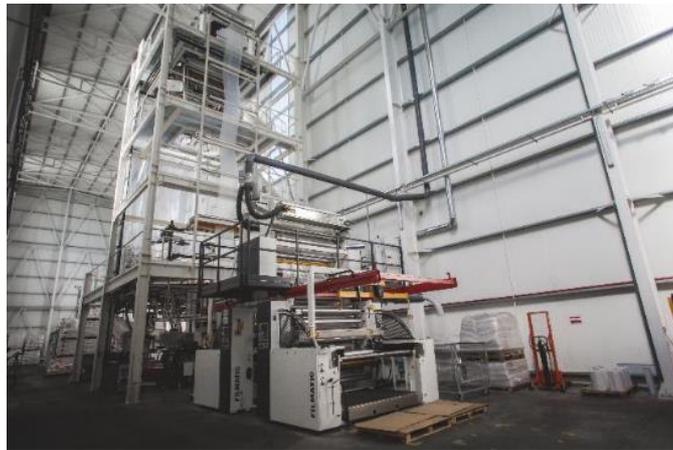
Figura 22 - Extrusora “Blow2” (Rembalcom, 2015)
