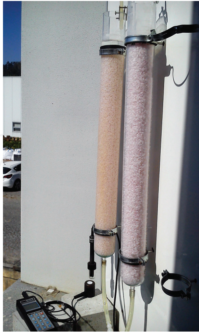
Figure 3. Filtration columns with a quartz porous media for OTC photo-oxidation.
