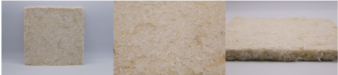
Fig. 6: Composite materials with chicken fibres reinforcing epoxy resin
