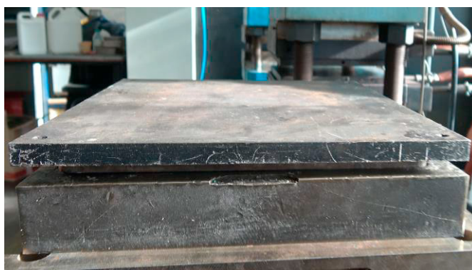
Fig. 1: Moulding compression equipment and mould used
