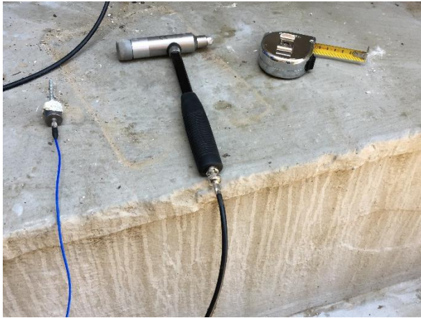
Figure 4-18 Equipment for sonic test: uniaxial accelerometer, hammer, ruler (from left to right)
