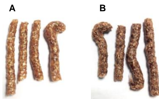
Figure 25 | Colour and roughness intensification with increasing residue contents. Polypropylene with 10 wt.% (A) and 20 wt.% (B) of wood flour.
