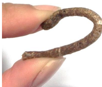
Figure 32 | Deformation observed on the mixture polyethylene with 20 wt.% of wood flour and 20 wt.% of plasticizer, when maximum flexural force was applied.
