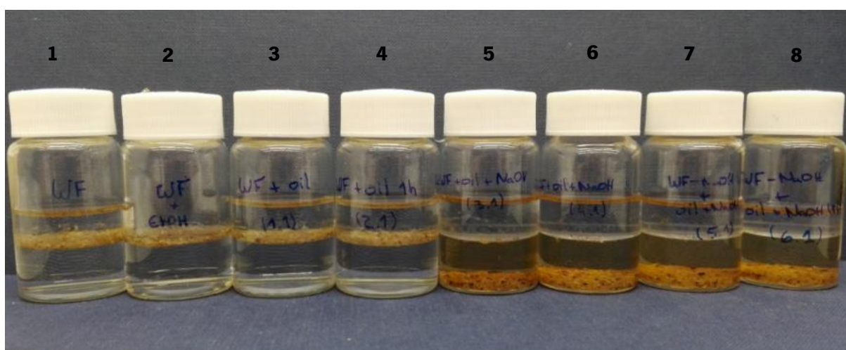
Figure 47 | Compatibility of wood flour samples, treated with different soybean oil solutions, for non-polar solvents. All samples were added to heterogeneous solutions with two immiscible solvents: water and petroleum ether. The number on each sample were attributed as follows:
