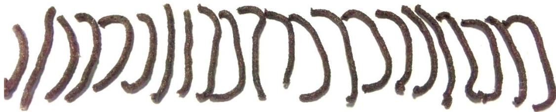
Figure 29 | Composition of mixtures obtained with plasticizers supplementation, by laboratorial scale extrusion. The represented filaments correspond to the mixture of polyethylene with 20 wt.% in content of wood flour and 10 wt.% of Durasyn 180.
