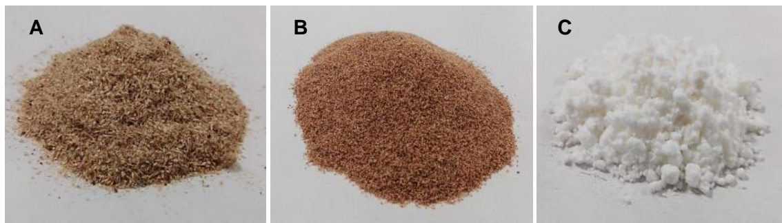
Figure 20 | Industrial forest residues used as bio-based reinforcing phases in the preparation of composites: Wood flour (A) , cork powder (B) , and cellulose fibres (C) .
