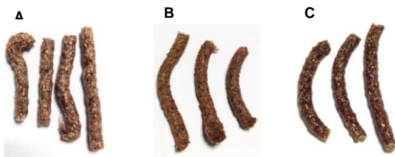
Figure 26 | Roughness of mixtures with 20 wt.% of wood flour and the three polymer basis: polypropylene (A) , polyethylene (B) and polylactic acid (C) .
