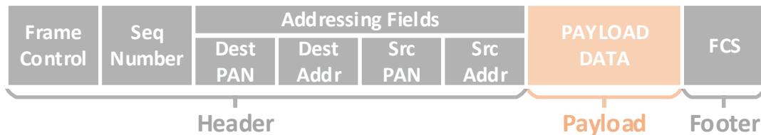
Figure 4.1: General IEEE 802.15.4 Data frame type.
