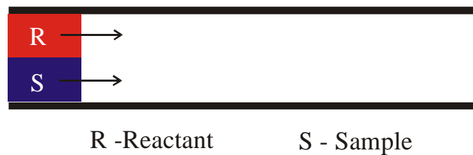
Figure 3 - In a uniaxial flow mixing between two parallel streams results exclusively from transversal diffusion.
