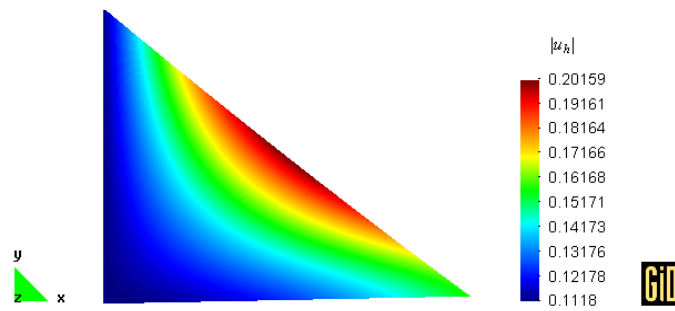
Figure 3.18: Problem 3 : the displacement field |u_h| for the mesh presented in Figure 3.17
