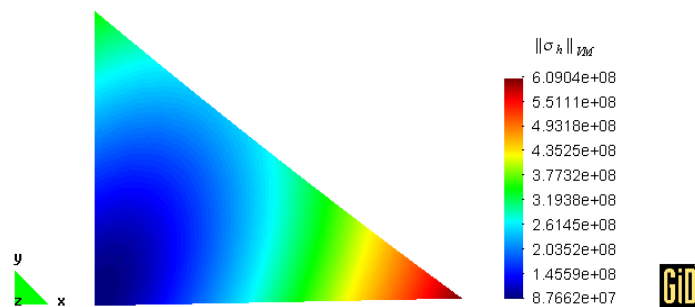
Figure 3.20: Problem 3 : the von Mises stress field for the mesh presented in Figure 3.17
