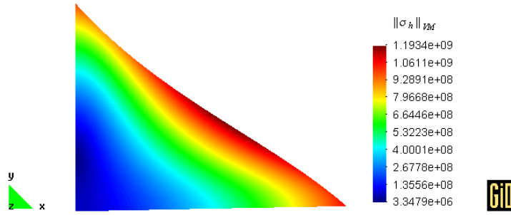
Figure 3.28: Problem 4 : the von Mises stress field for the mesh presented in Figure 3.25
