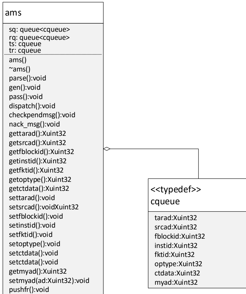
Figure 4.21: Application Message Exchange Service Software Architecture
