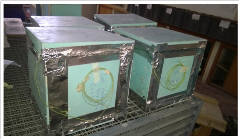
Figure 1. Small-scale test cells used for the thermal efficiency characterization.
