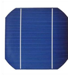
Figure 2.18 - Monocrystalline solar cell [39].
