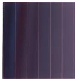
Figure 2.20 - Amorphous thin film solar cell [39].
