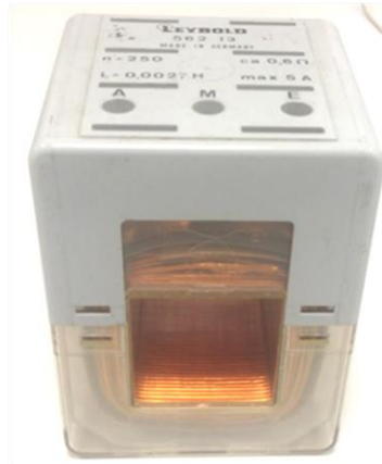
Figure 5.17 - Inductor used for the DC-DC converters.
