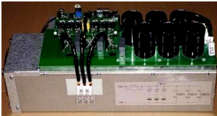
Figure 5.13 - PowerSys P3G lab converter module used in the power converter prototype.
