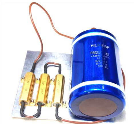
Figure 6.18 - RC load used to simulate the charging of the battery.
