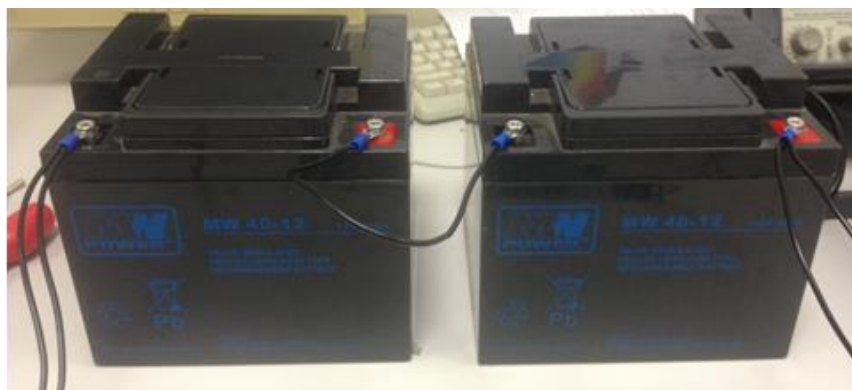
Figure 5.18 - MW 40-12 batteries used in the power converter prototype.
