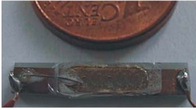
Fig. 5. The 1 st prototype tunable Fabry-Perot optical filter.
