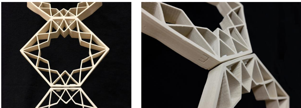
Figure 7. Inclusion of connection elements in other materials (PLA).
