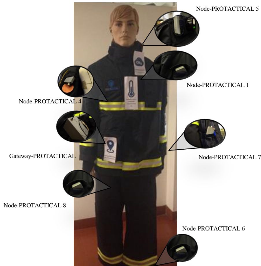
Figure 4.4. PPE prototype with several Edge of the Network nodes integrated into/onto the textile subsystem.
